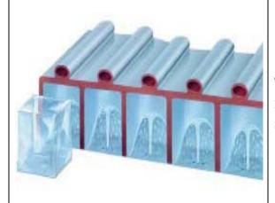
The ABS water plate sprays water up into the evaporator cells to form the square IM cube.
